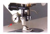
EXTREMELY CLOSE PULLING, FACILITATES CURVE AND SHORT SEWING ON THIN MATERIALS.
